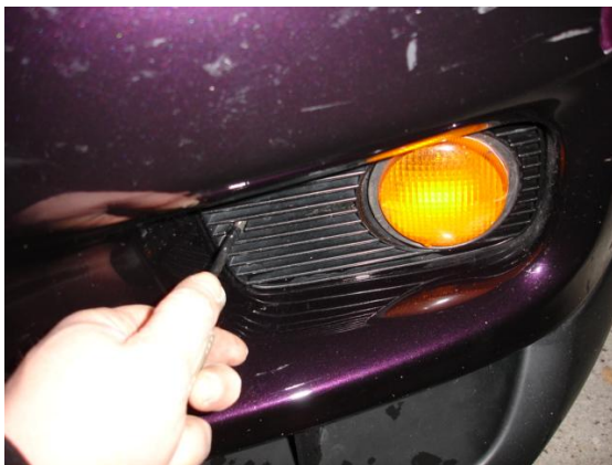
Remove indicator to get at hidden headlamp bolt
