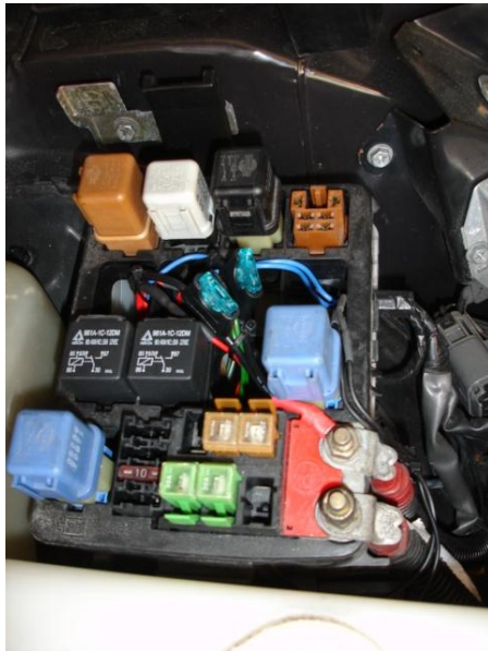
Relays and fuses neatly installed in engine bay relay/fuse box
