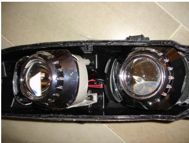
Trial assembly - showing shutter actuator wires in place, adequate clearances between shrouds and housing
