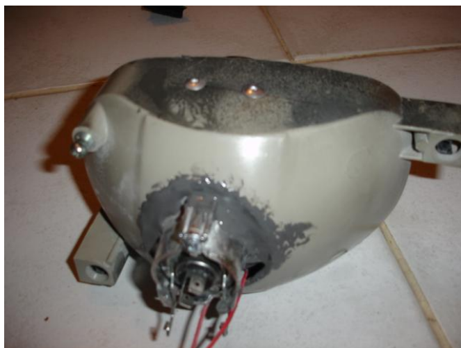
Glued and riveted unit – rear view. Note grey JB Weld putty filling the gap between the hole cut in the reflector and the projector
