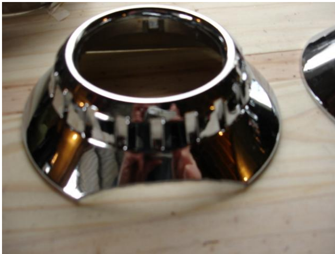
Cut shroud, ready to glue in place
