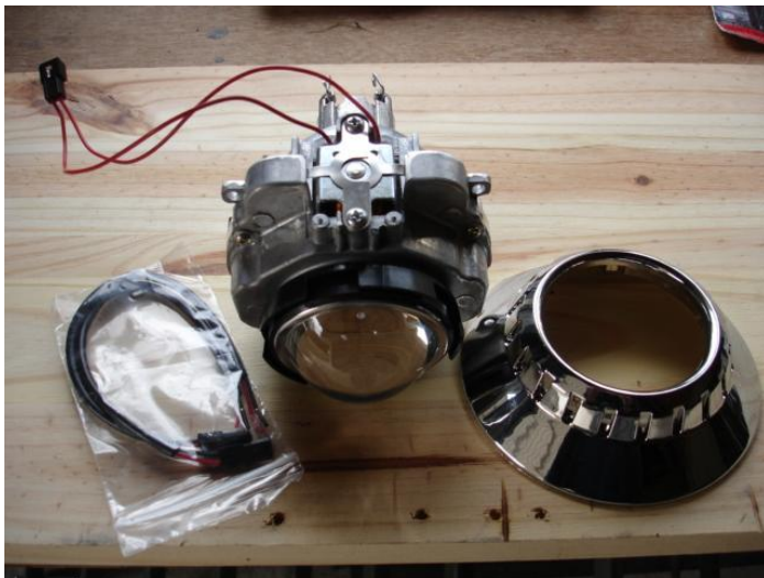
FX-R projector units with shroud and cable kit for high-beam shutter actuation
