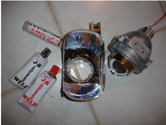
Ready for gluing...note surfaces keyed to aid adhesive bond
